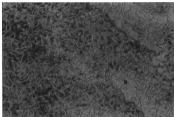
Figure 6. Polarized optical micrograph (200 \times ) observed after annealing poly{5-[[11'-(2'',5''-bis[2-[(3'-fluoro-4'- n -heptoxyphenyl)ethynyl]phenyl]undecyl]oxy]carbonyl]bicyclo[2.2.1]hept-2-ene} at 43.2 °C for 16.5 h upon cooling from the isotropic melt; 43.2 °C, schlieren nematic texture.
